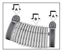
2. Insert the anti-static wire through the flexible pipe.
