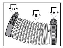
2. Insert anti-static wire through flex tube.
