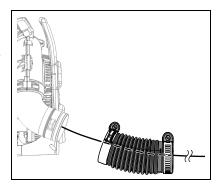
3. Assemble flexible pipe to elbow (D) on blower. Position clamp with cable guide loop (G) on outside of flexible pipe and tighten clamp.
