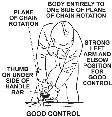
**⚠ WARNING!** Do not thrust the nose of the saw into a pile of branches or dense brush where you cannot see whether the nose is in the clear. A high risk of kickback exists under such conditions. **INSTALL THE OPTIONAL KICK GUARD™ DEVICE** before attempting such applications.
