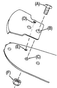
**Use the optional Kick Guard in cutting applications where the bar's tip may come into contact with solid objects or surfaces. Most cutting operations can be accomplished with the optional Kick Guard in place.**
