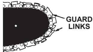
The low-kickback saw chain on your saw has depth gauges and guard links to reduce kickback. Depth gauges control the depth of cut. The guard links help to prevent the cutters from digging in too deeply at the bar nose. Low-kickback chain tends to resist penetration of the bar tip, which is the cause of kickback; however, the chain may "skate" along the surface of the wood. Skating the nose bar into an obstruction could result in a kickback.
