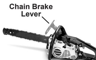
**⚠ WARNING!** It is the responsibility of the owner or operator to ensure that the brake is serviced, adjusted, and tested in accordance with the instructions as detailed in your instruction manual in order to ensure that the brake performance is maintained in compliance with ANSI B175.1- 2000, which stipulates that the brake shall stop the chain in a maximum of 0.15 seconds after activation (0.12 Average).
