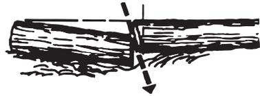
**MAKE ANGLED CUT WHEN ONE SECTION MAY SETTLE AGAINST ANOTHER. KEEP BODY OUT OF BAR/CHAIN PATH!**
