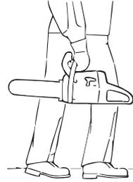
**CARRY SAW WITH BAR TO REAR & ENGINE STOPPED**
