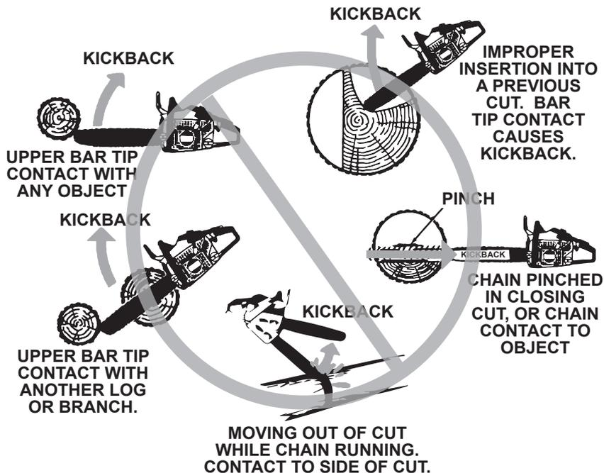
⚠ **WARNING!** Hold the saw firmly with both hands. Make sure your left thumb is always on the underside of the front handle. Never over the top! Keep your left arm straight with the elbow locked to prepare for any sudden or unexpected reaction of the chain saw, and to maintain better control.
