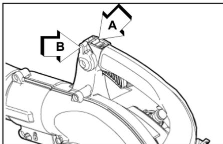
**Note:** Engine will not run if safety switch is not activated.
