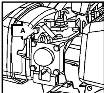
3. Check idle speed and reset if necessary. If a tachometer is available, idle speed screw (A) should be set to the specifications found on “Specifications” Page of this manual. Turn idle screw (A) clockwise to increase idle speed; counterclockwise to decrease idle speed.
