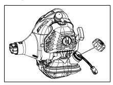
Note: Federal EPA regulations require all model year 2012 and later gasoline powered engines produced for sale in the United States to be equipped with a special low permeation fuel supply hose between the carburetor and fuel tank. When servicing model year 2012 and later equipment, only fuel supply hoses certified by EPA can be used to replace the original equipment supply hose. Fines up to \$37,500 may be enforced for using a non-certified replacement part.
