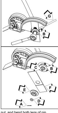
6. Install new split pin (A) to secure nut, and bend both legs of pin counterclockwise around PTO shaft (C).
