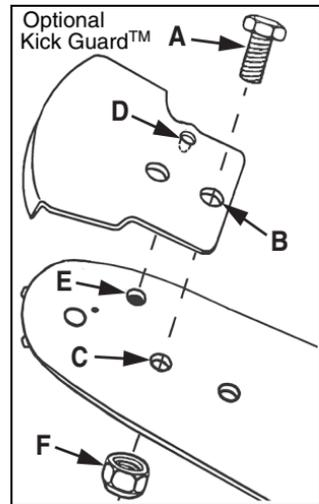
**Guide Bar and Saw Chain Installation / Removal**
