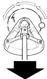
As shown in the illustration, a blade turning counterclockwise will cause the equipment to pull away from the operator if the point of cutting resistance is on the left side of the blade. If the point of cutting resistance is on the right side of the blade, the equipment will push back toward the operator. In both examples, the reactive force is in the opposite direction of blade rotation at the contact point where resistance occurs.
